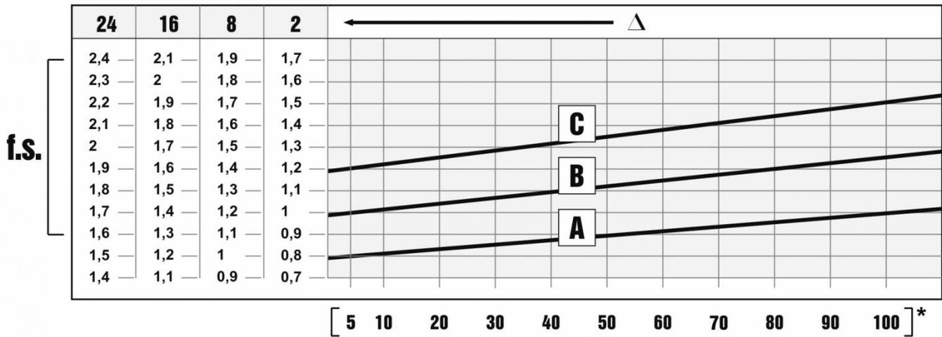
The service factor (f.s.) depends on the operating conditions the gear reducer is subjected to.
